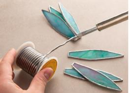
STEP 5: Turn leaves over (onto points) and fill in base with solder. Cut 2" dowel, wrap it in copper tape, and brush it with safety flux. Then solder it to base of succulent. Tin rest of dowel.
